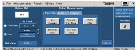
8. Select Measurement > Select > Transmitter > Eye Diagram. (Alternatively, in the Transmitter tab, select the Eye Diagram measurement.)
